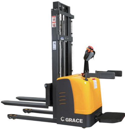
CDD Series Full Electric Pallet Stacker CDD10/15/20 -Load 1000/1500/2000KG -Load center distance 500MM -Drive motor power 1.5KW -Increase motor power 2.2KW -Electromagnetic brake -Optional distribution steering PAGE11
