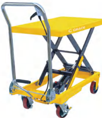
SDP Series 150/300/500kg Manual Platform Truck SDP150/300/500 -Load 150/300/500KG -Lifting height 515/620/590MM -Maximum height 740/900/900MM -Body length 700/942/1670MM -Wheel diameter 100/127/127MM PAGE22
