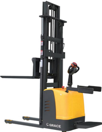
CDD Series High Lift Full Electric Pallet Stacker CDD10/15/20 -Load 1000/1500/2000KG -Load center distance 500MM -Drive motor power 1.5KW -Increase motor power 2.2KW -Electromagnetic brake -Optional distribution steering PAGE13
