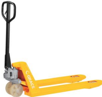
BD Series 2000/3000kg Manual Pallet Truck BD -Load 2000/3000KG -Lifting height 190MM -Overall length 1520/1590MM -Turning radius 1265/1335MM -Self weight 70KG PAGE21
