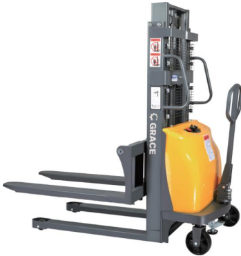
BDD Series Semi-electric Stacker BDD10/15/20 -Load 1000/1500/2000KG -Load center distance 500MM -Overall length 1860MM -Increase motor power 1.6KW -Mechanical brake PAGE7
